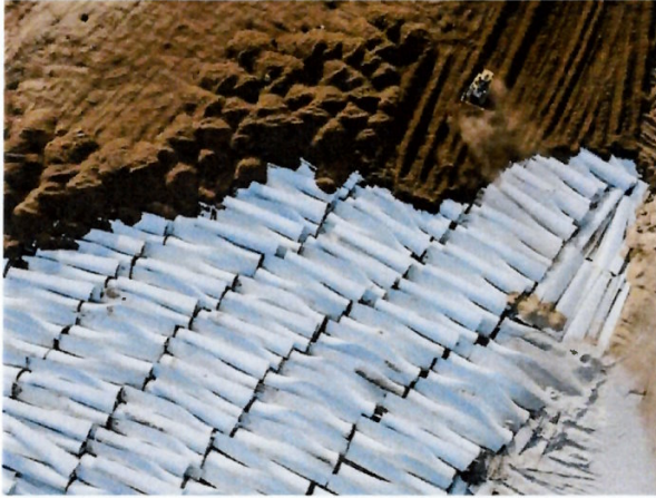
Figure 12: Fragments of wind turbine blades await burial at the Casper Regional Landfill in Wyoming (Source: https://www.bloomberg.com/news/features/2020-02-05/wind-turbine-blades-can-t-be-recycled-so-they-re-piling-up-in-landfills )
